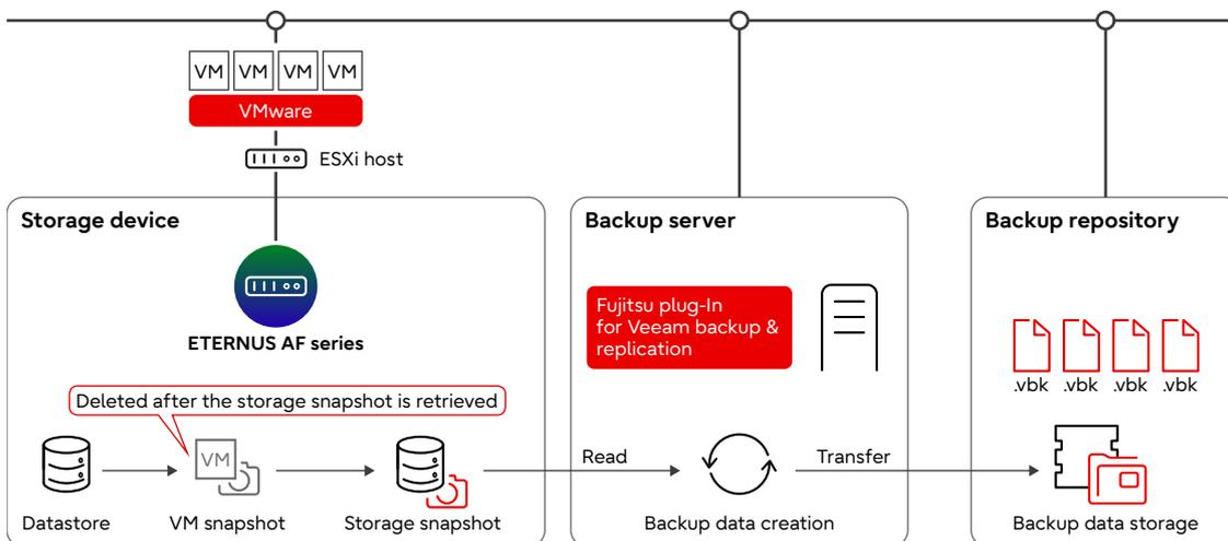
The storage snapshot is saved and is read in a separate area of the storage system from the datastore and VM snapshot. The VM snapshot is automatically deleted after the storage snapshot is completed. Then, the storage snapshot is automatically deleted after the backup is completed.
