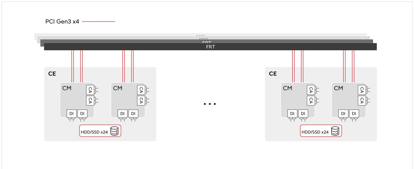
Figure 8: Schematic illustration of Controller Enclosures – all components in the enclosures are hot-pluggable.
