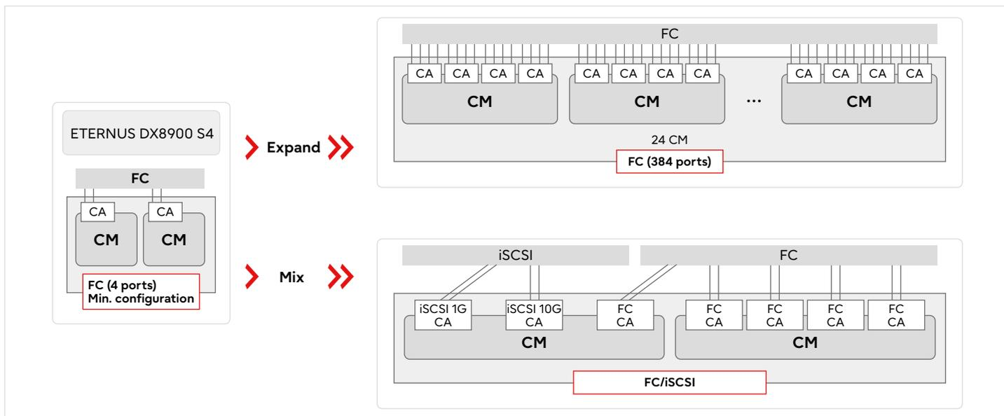
Figure 7: All types of Channel Adapters can be mixed on a Controller Module.
